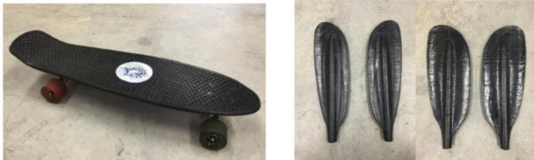
Figure 14. A skateboard and paddle for kayaks realized using 3D printing. Source: Byard et al., 2019)
